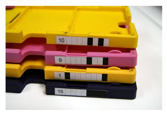
For correct operation, labels have to be accurately placed in the specific position. The first black line on the right of the number must be aligned with N-E divider on the board:
