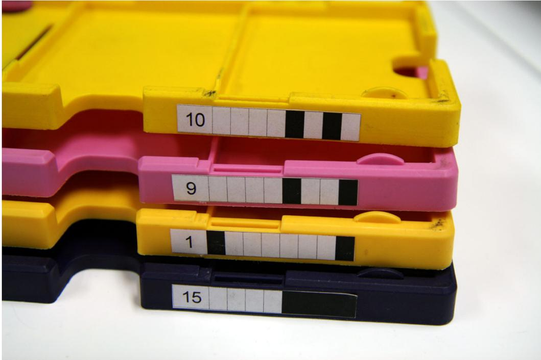
For correct operation, labels have to be accurately placed in the specific position. The first black line on the right of the number must be aligned with N-E divider on the board:
