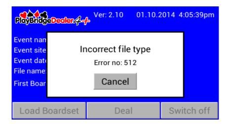
In the case of any loading errors, the Dealer4+ returns to the Main Screen. If the right file is selected but is corrupted or has an incorrect format, more specific information about the problem is displayed - for example:
