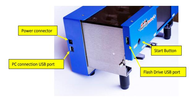
The machine does not have a power switch. To turn it on - press and hold the START button on the front panel of the machine for 2 seconds. It is possible to turn off the machine via a button on the Main Screen of the Front Display.
