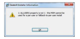
This error happens only during updating from version 4.34 or earlier. This is because of a bug in the previous version. At this point the previous version is uninstalled but installation of the new version cannot continue automatically. Click OK.
