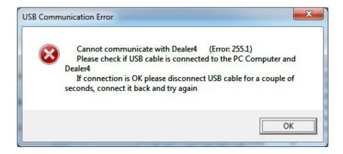
To resolve this problem, uninstall and install software again. If this does not help manual USB driver installation maybe required.
